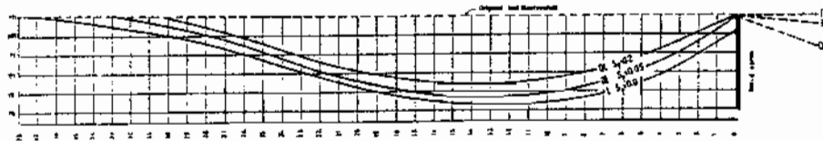
Fig.4- Scour hole profiles with the change of the adverse slope of the rear apron
