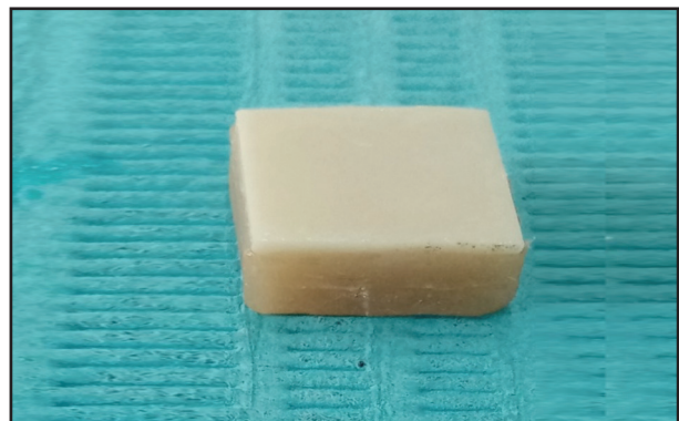
Figure (1): Ceramic veneer cemented to composite resin substrate
