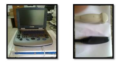
**Fig. 1:** An ultrasound machine (EXAGYN ECM company, France) (the left). A micro convex probe 3.5-5 MHz and a linear array probe 6-8 MHz (the right).
