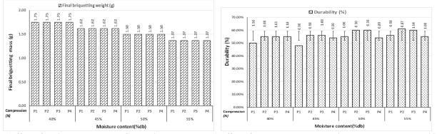
c)Effect of moisture content on final briquette mass d) Effect of pressure value and moisture content on durability Fig.7. Briquetting quality for the dried chamomile petals ray flowers
