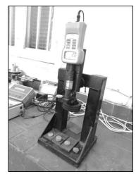
Fig .3. An image for the manual briquetting device
