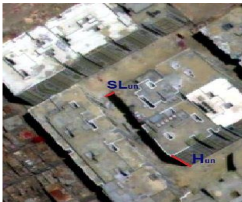
Figure 9. The height and shadow length of an unknown building
