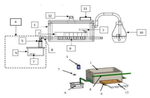
**Fig 1.** The thermochemical poultry egg incubator prototype components,1- The incubator frame, 2-eggs tray, 3- turning motor, 4- material humidification unit, 5- fan,6- water tank, 7- ultra-sonic humidifier, 8- vapor pipes (perforated pipes), 9- storage material container (TCMs), 10- humidifier for incubator atmosphere, 11,12- display for temperature and humidity,13- Aluminum sheet
