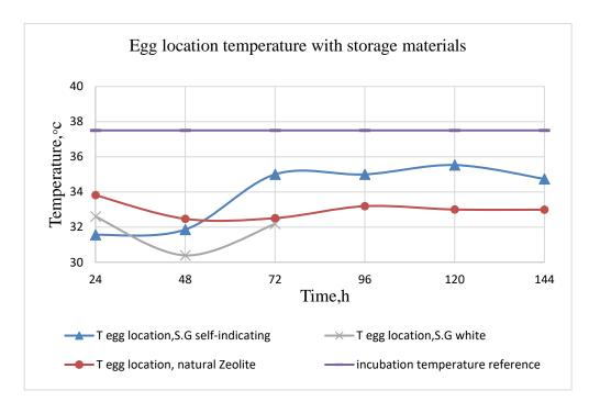
**Fig 14.** The egg location temperature with storage materials (Silica gel self-indicating, Silica gel white, Natural Zeolite)
