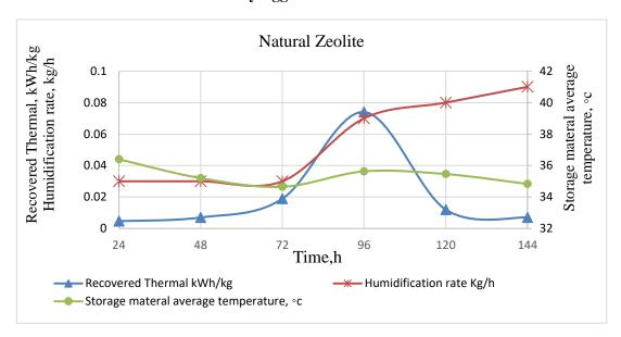
Fig 11. The recovered thermal and temperature of storage material with the humidification rate of storage material (Natural Zeolite)
