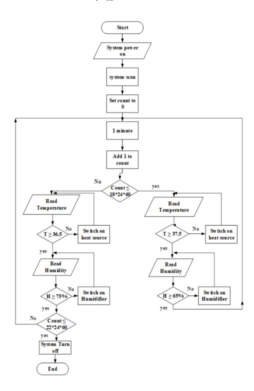
Fig 4. The control of the temperature and humidity inside the thermochemical poultry egg incubator flowchart
