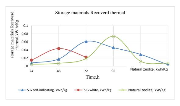
**Fig 8.** Illustrate the recovered thermal, in (kW.h/kg) of storage materials (Silica gel self-indicating, Silica gel white, and Natural Zeolite) during the time
