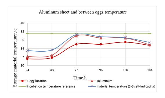
**Fig 15.** The average temperature for aluminum sheet and eggs location with storage material Silica gel self-indicating
