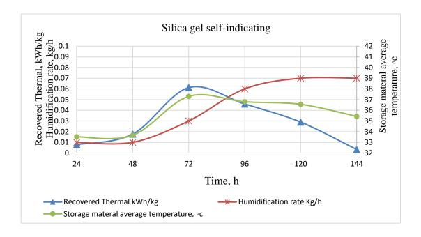
**Fig 9.** The recovered thermal and temperature of storage material with humidification rate of storage material (Silica gel self-indicating)
