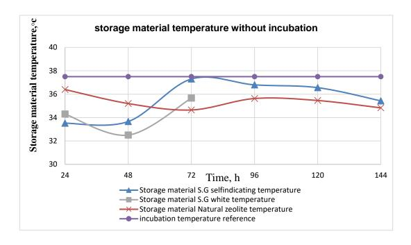
Fig 13. Storage material temperatures during recovered thermal process and incubation temperature
