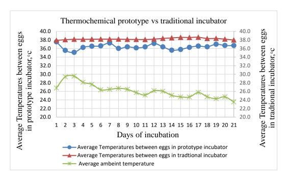
Fig 16. The average of temperature between eggs in thermochemical prototype and traditional incubator
