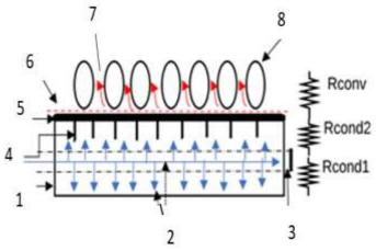
**Fig 7.** Illustration of the process of recovering thermal process and heat transfer from TCM to the aluminum sheet to eggs where: - 1- the storage material container, 2- vapor flow, 3- perforated vapor pipes, 4- fins, 5- aluminum sheet, 6-the egg tray, 7- heat flow, 8- egg
