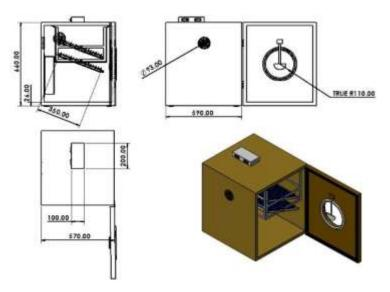
Fig 5. The traditional poultry egg incubator
