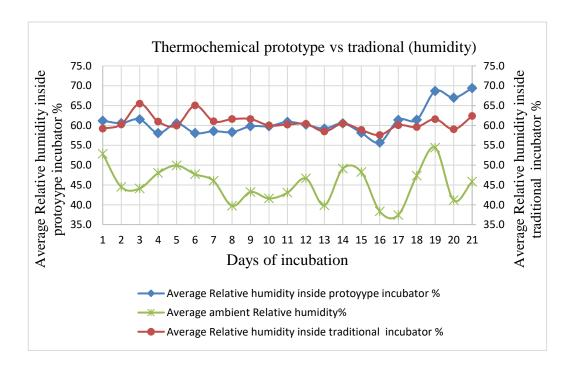
Fig 17. The average relative humidity inside the thermochemical prototype and traditional incubator
