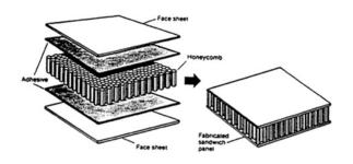
Figure(5) honeycomb sandwich panel
