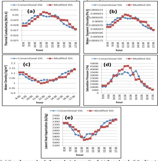
Fig. 5. Variations of average hourly thermo-physical properties of: (a) thermal conductivity, (b) water dynamic viscosity, (c) water density, (d) saturation pressure and (e) latent heat of evaporation, for both conventional and modified SSSs.
