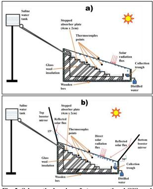
Fig. 2. Schematic drawing of a) conventional SSS, and b) modified SSS.
