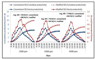
Fig. 6. Variations of hourly and cumulative distillate water productivity for both conventional and modified SSSs at different salinity levels.
