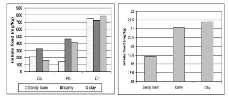
Fig. 1. Initially fixed heavy metal concentrations in the artificially contaminated soils.
