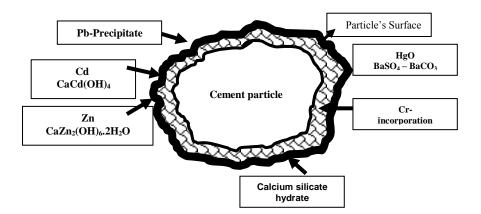
Fig. 6. Immobilization of heavy metals by hydrated particle of Portland cement as suggested by Ganjidoust *et al.* (2009).
