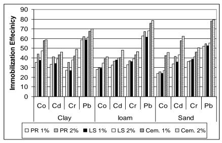
Fig. 5. The efficiency of the heavy metals immobilization for different types and rates of local amendments.
