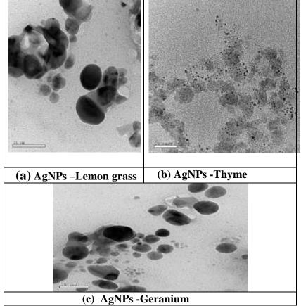
Fig., (3a, b&c) : Transmission electron microscope (TEM) image of AgNPs synthesized by (a) Lemon grass, (b) thyme & (c) geranium.
