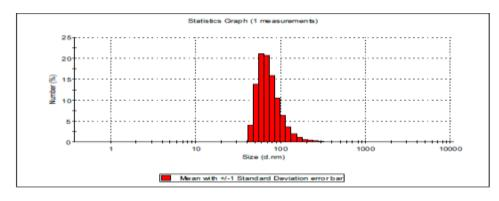
Fig., (2c): Dynamic light scattering (DLS) of AgNPs synthesized by geranium P. graveolens.
