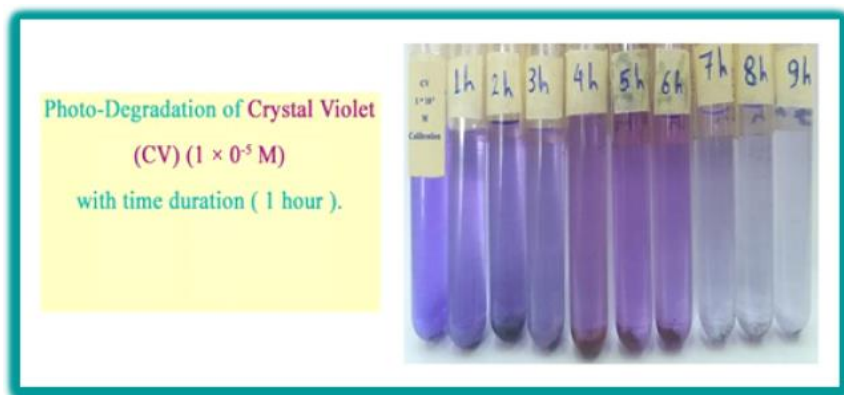
Fig. 7 Gradual photo-degradation and decolourization of Crystal Violet (CV) dye ( 1 \times 10^{-5} \text{ M} ) with time duration 1 hour utilizing \text{Ni}_{0.1}\text{Co}_{0.9}\text{Fe}_2\text{O}_4 Nano-spinel as photo-catalyst.
