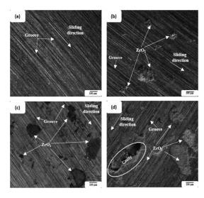
**Figure 11** Optical micrographs of worn surfaces of AlMg5/ZrO<sub>2</sub> composites with different  $ZrO_2$  contents. (a) 0, (b) 5, (c) 10, and (d) 15 wt.%  $ZrO_2$ .
