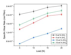
**Figure 9** Effect of applied load on the specific wear rate of AlMg5/ZrO<sub>2</sub> composites.
