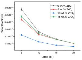
**Figure 10** Effect of applied load on the wear coefficient of AlMg5/ZrO<sub>2</sub> composites.
