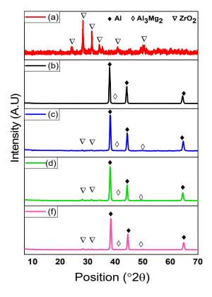
Figure 4 XRD patterns of  $ZrO_2$  and AlMg5 with different  $ZrO_2$  particles content. (a) $ZrO_2$  powders, (b) AlMg5, (c) AlMg5/5 $ZrO_2$ , (d)AlMg5/10 $ZrO_2$ , and (f)AlMg5/10 $ZrO_2$ .
