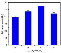
**Figure 6** Effect of ZrO<sub>2</sub> particles content on the hardness of AlMg5/ZrO<sub>2</sub> composites.
