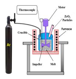
Figure 1 A schematic diagram for stir casting aperture.
