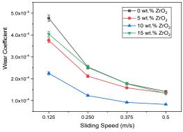
**Figure 8** Effect of sliding speed on the wear coefficient of AlMg5/ZrO<sub>2</sub> composites.
