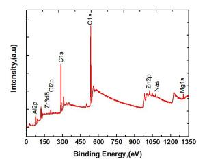
Figure 14 The representative XPS spectra analysis (survey scan) of AlMg5/10ZrO₂ composite worn surface.
