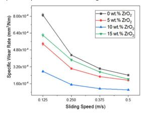
**Figure 7** Effect of sliding speed on the specific wear rate of AlMg5/ZrO<sub>2</sub> composites.
