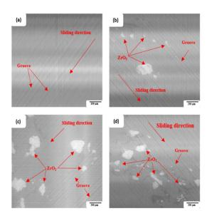
Figure 12 SEM images of worn surfaces of AlMg5/ZrO<sub>2</sub> composites with different  $ZrO_2$  contents. (a) 0, (b) 5, (c) 10, and (d) 15 wt.%  $ZrO_2$ .
