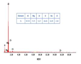
Figure 13 EDS analysis of AlMg5/10ZrO $_2$  composite worn surface.
