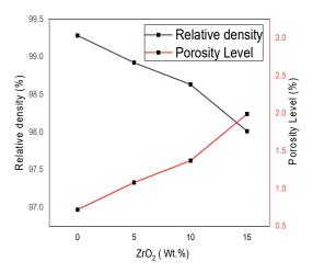
Figure 5 Effect of ZrO<sub>2</sub> particles content on the relative density and porosity level of AlMg5/ZrO<sub>2</sub> composites.
