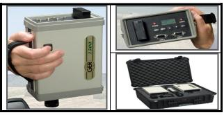
Plate (2): Field Portable Hyperspectral Radiometer (FPHR): Model- GER 1500
