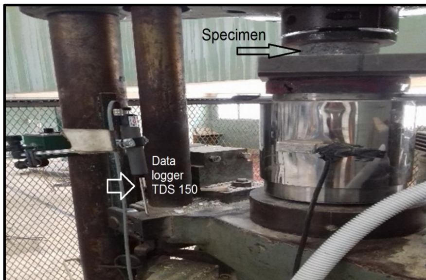
Figure 1. Aquasi-static test with universal testing machine & max load 30 ton
