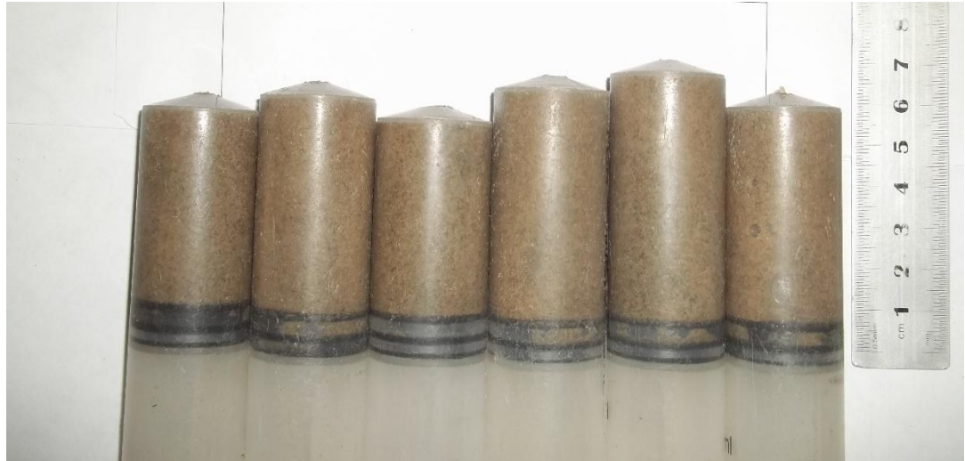
Fig. 1. Measurement for oxidic-anoxic layer in the experimental tanks using soil core.
