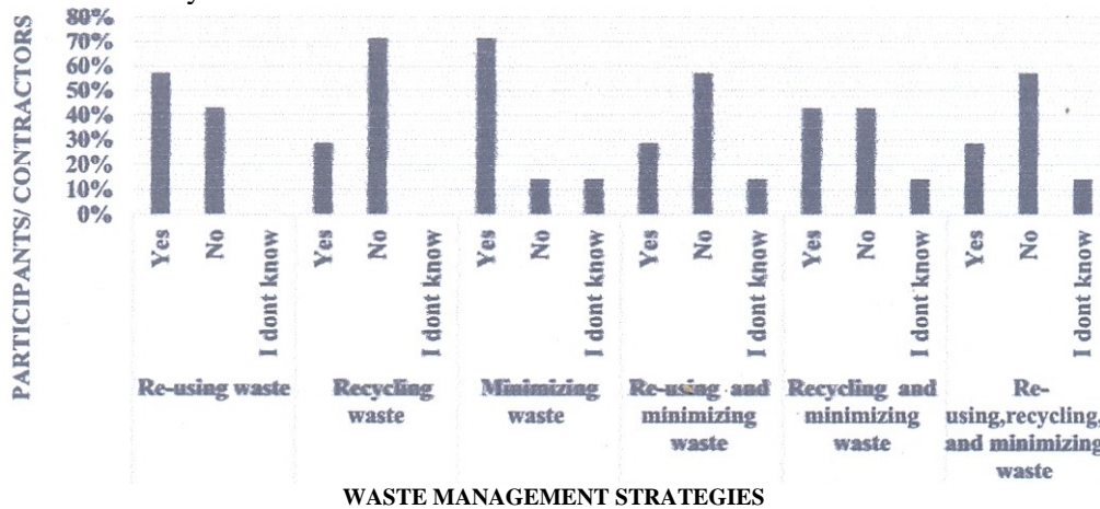
Fig.6- Using of waste management strategies by contractors in Egypt (source: researcher)
