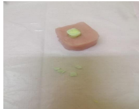
Figure 4 : Fracture of occlusal ceramic veneer
