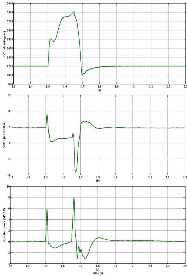
**Fig. 11** Performance of studied system in case of stator series crowbar technique.
