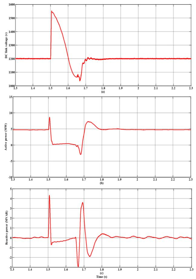
**Fig. 10** Performance of studied system in case of traditional rotor crowbar technique.
