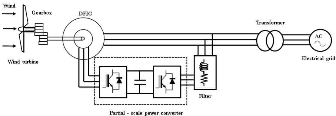
**Fig. 2** Variable speed DFIG-WT with partial-scale power converter.
