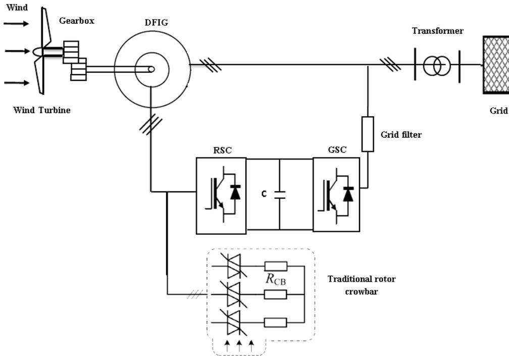
**Fig. 4** Diagram representation of DFIG-WT operated with traditional rotor crowbar circuit.
