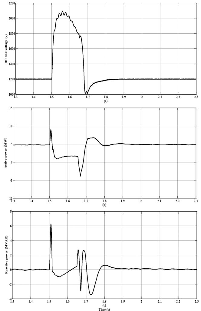
**Fig. 8** Performance of studied system in case of without crowbar technique.
