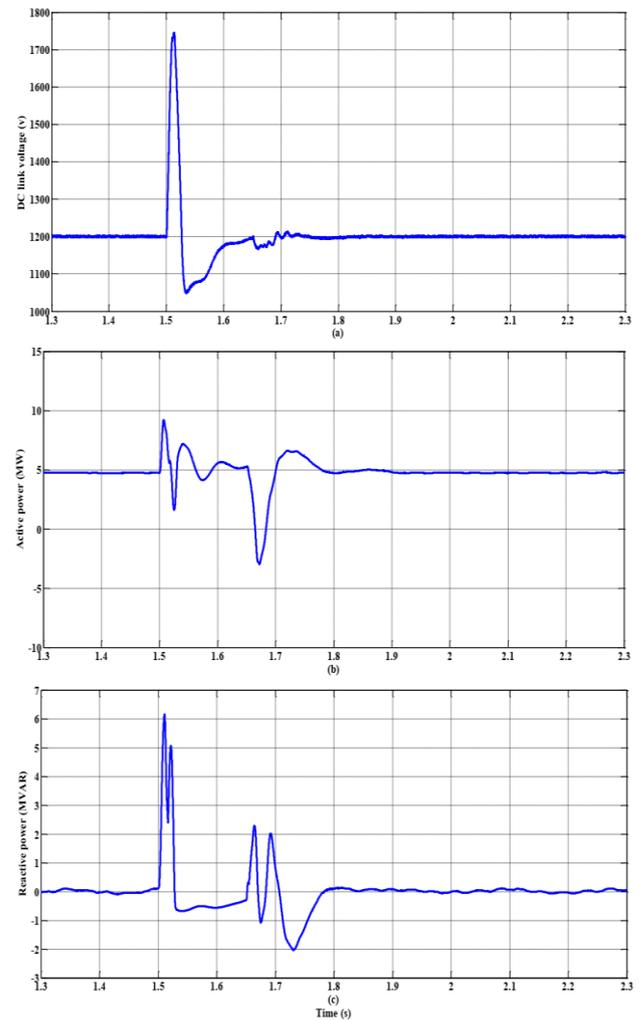
**Fig. 12** Performance of studied system in case of outer terminal crowbar technique.
