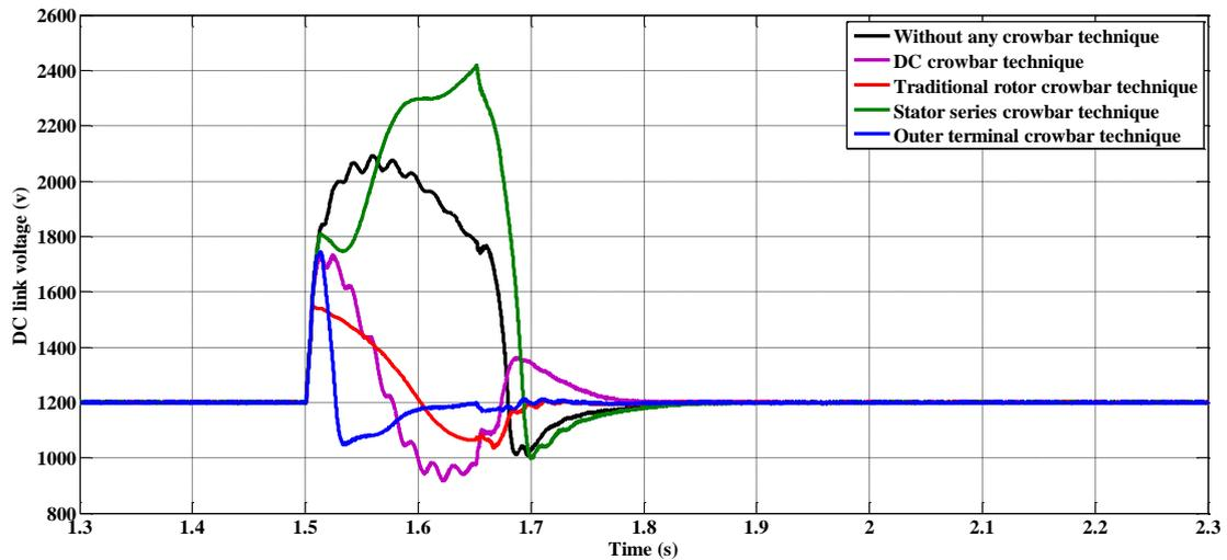
**Fig. 13** Comparison of DC link voltage responses during different crowbar techniques.
