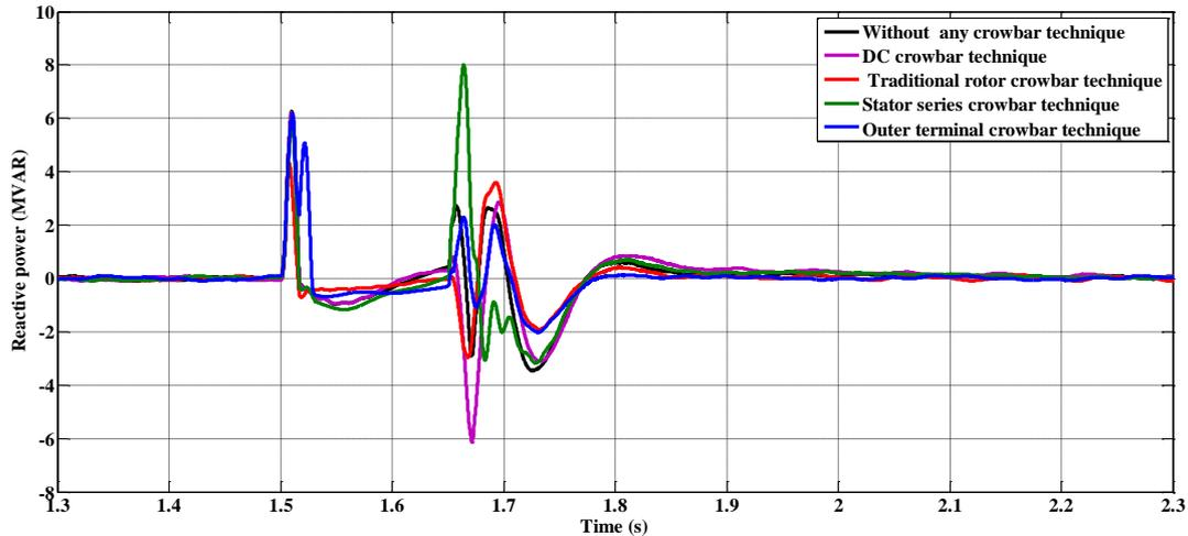
**Fig. 15** Comparison of reactive power responses during different crowbar techniques.
