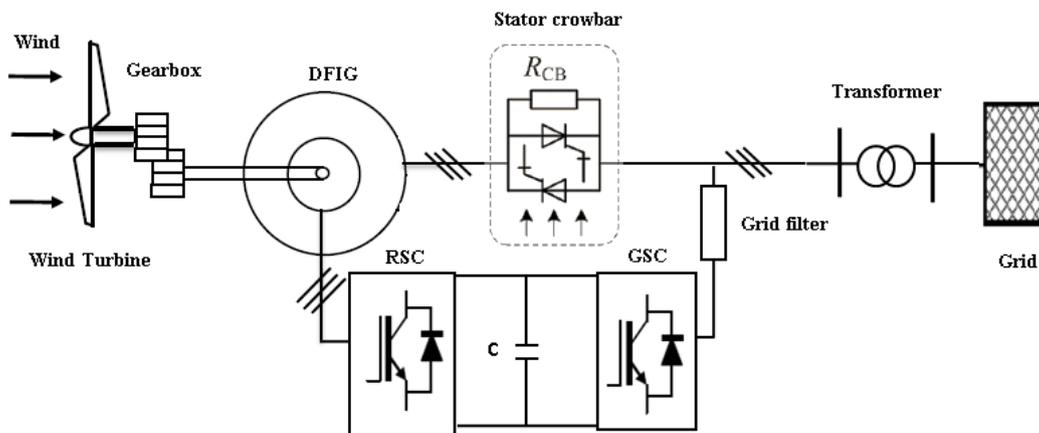
**Fig. 5** Diagram representation of DFIG-WT operated with stator series crowbar circuit.
