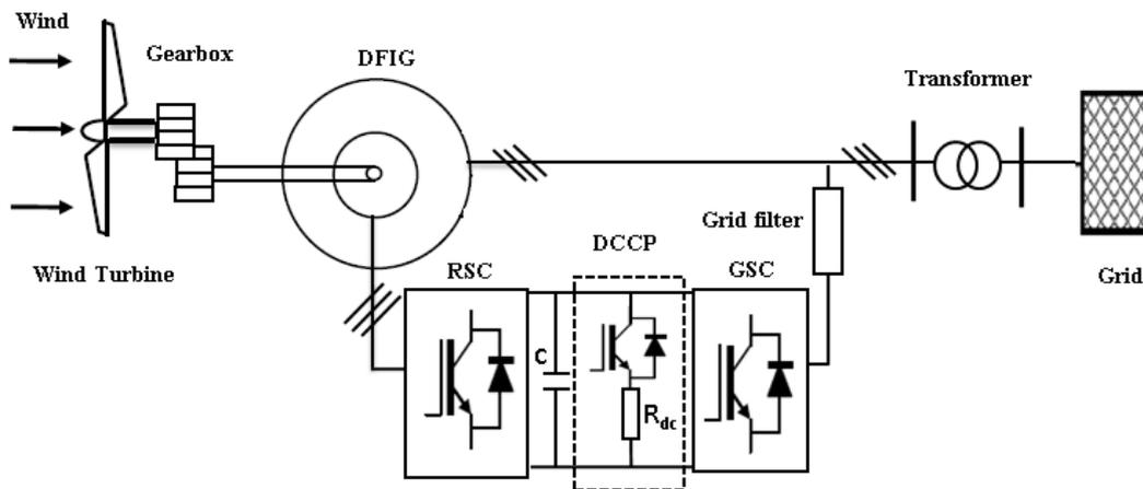
**Fig. 3** Diagram representation of DFIG-WToperated with DCCP circuit.
