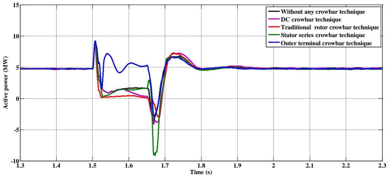
**Fig. 14** Comparison of active power responses during different crowbar techniques.
