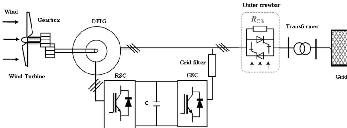
Fig. 6 Diagram representation of DFIG-WT operated with outer crowbar circuit.
