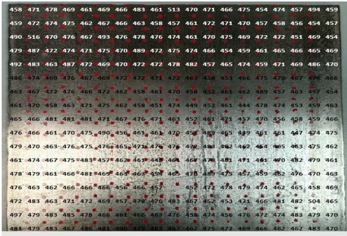
Fig. 8 The hardness map among the armor steel sheet.
