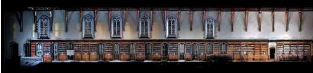
Figure 33. As part of the conservation plans as well as providing a quick snapshot at the time, the laser scanning was used to create the detailed geometry and horizontal projections of the cathedral then determined the process of processing the church. A three-dimensional laser scan was performed over 10 days in the cathedral using a FaroPhoton120 laser scanner (Figure 34).
