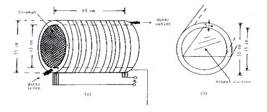
Figure (3-1) Magnetic field generator
