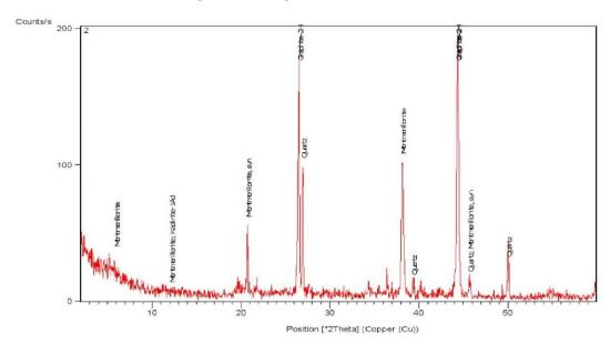
Fig. 7. XRD analysis of adobe blocks (Amenemhet III pyramid)
