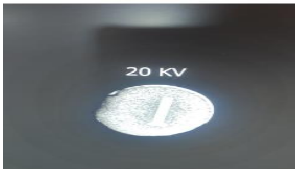
Fig. (5) Show penetration of X-ray for sample rubber composite with 100 pphr TiO 2 .
