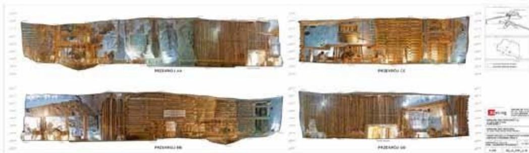
Figure 50. Sections of project after 3D Laser scanning application.
