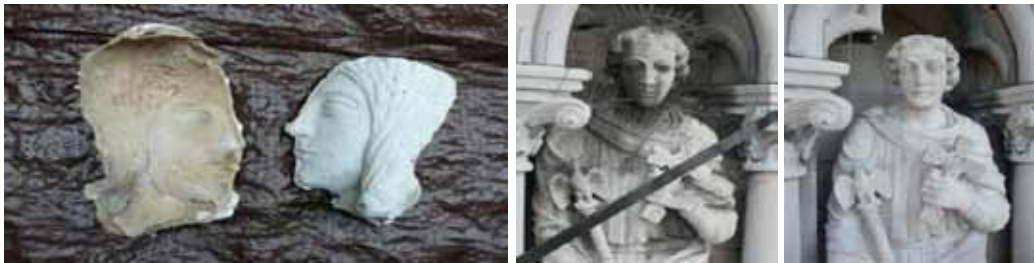
Figure 6. Modeling Replacement for Sculpture Losses, Sculpture Conservation, Face Replica. The project showed a hard shell formed on the outside of many sculptures, while the basic stone materials have been eroded leaving only loose grains. The cracks formed on the surfaces to expose the damaged interior to the water and caused the full elements to fall (Figure 7). Materials / Limestone, Mortar.
