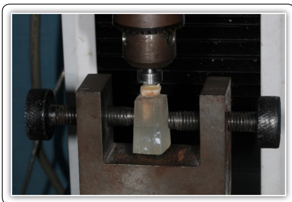
FIG (1) Mounting of the sample in universal testing machine for tensile test
