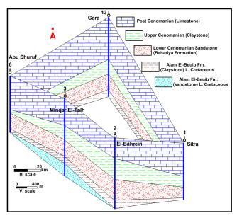
Fig (8): Panel diagram showing the subsurface configuration in East Siwa Oasis, Western Desert, Egypt.
