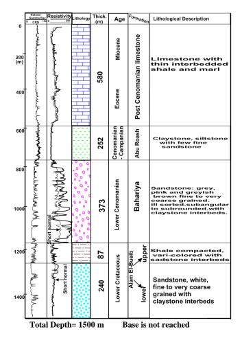
**Fig** (2): Composite lithostratigraphic section and geophysical logs of well no. 3 (modified after <sup>[5]</sup>).
