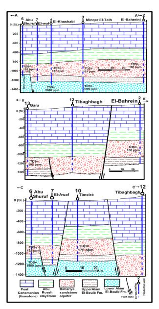
**Fig (9):** Hydrogeological cross-sections, East Siwa Oasis area.
