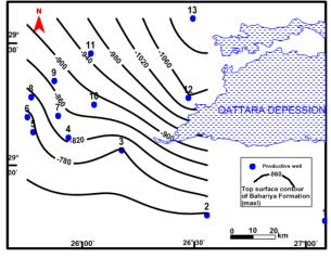
**Fig** (4): Structure contour map of top surface Bahariya sandstone Formation.
