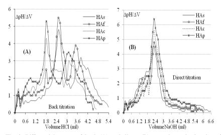
Fig. 2. Differential curves of back (A) and direct (B) potentiometric titration of humic acids isolated from alluvial soil (HAs), farmyard manure (HAf), compost (HAc) and poudrette (HAp).
