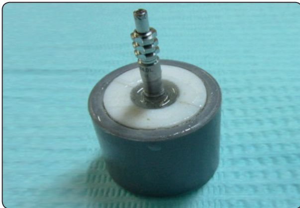
Fig. (1): Implant analog attached to impression copings, mounted vertically in resin block.
