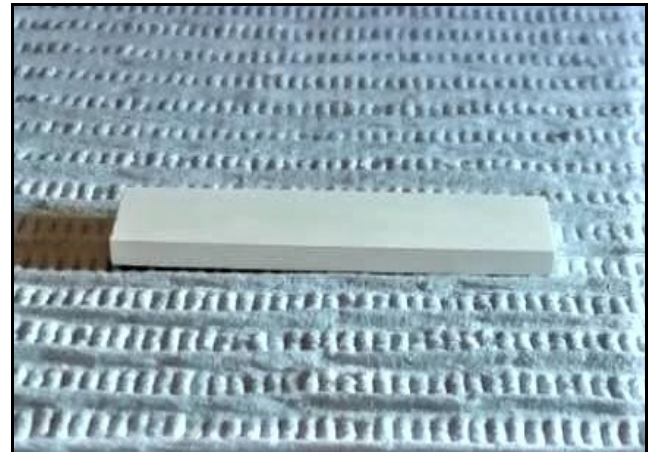
Figure (1): Showing a polished pre-sintered (Y-TZP) specimen.
