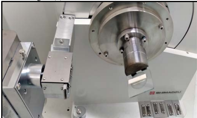
Figure (3): Showing (Y-TZP) bar specimen during X-Ray Diffraction test.
