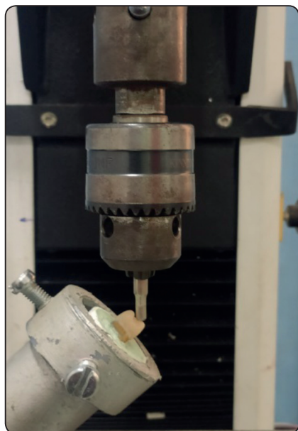
Fig. (2) Fracture resistance test with a Universal testing machine.
