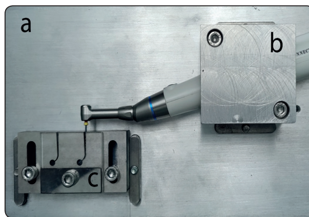
Fig. (1) Cyclic fatigue device showing: a: main frame, b: contra housing and endodontic contra inside, c: simulated artificial canal
