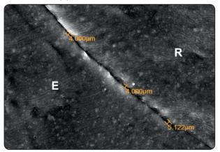
Fig. (3): SEM image at magnification x250 of inverse replica of (group I) restoration after one year follow up period showing micro gaps at interface between the restoration (R) & tooth enamel (E).
