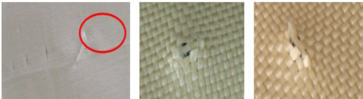
Fig.7. Cut behavior in silk fabric and para-aramid samples.
