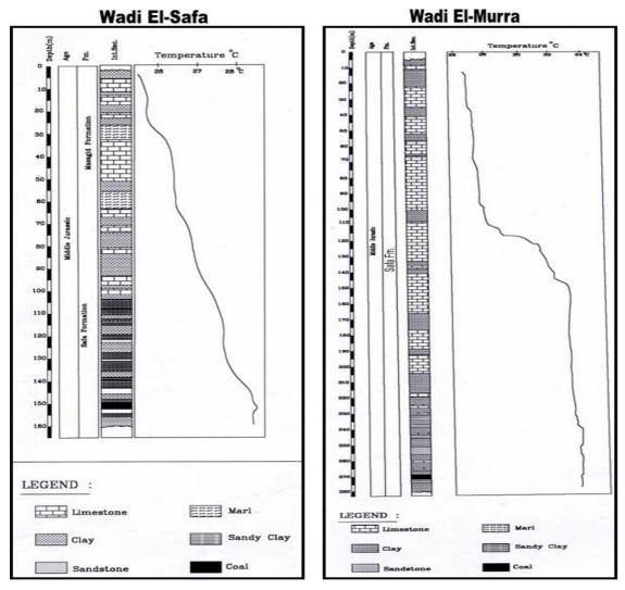
Figure (4): Temperature – Depth Curves at Wadi El-Safa B.H.No. 1 and Wadi El-Murra B.H.No. 9.
