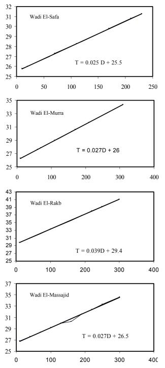
**Figure (5):** The relations between depth (m) and temperature (°C) of the study area.
