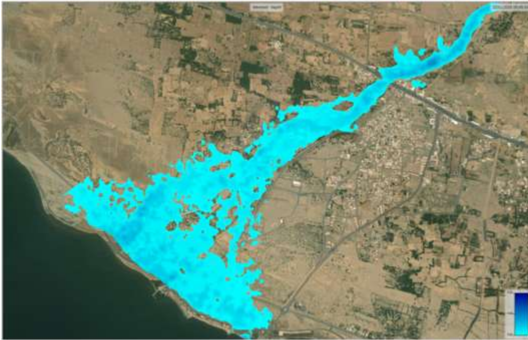
Fig. 16: Flood waters depth and flooded areas simulated by HEC-RAS2D model for 100-year of Reem.
