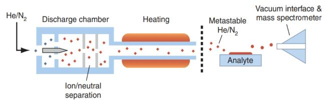
Figure 3: Direct analysis in real time for ambient analysis of samples without preparation. Reprinted with permission from (Cooks et al., 2006).
