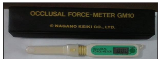
Figure (2): Occlusal force meter.
