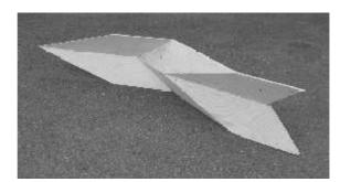
The prototype completed should pass the test showed important deformations of the structure particularly on the open sides. The results showed the importance of the connections in the proposed structures. The goal of the test is to improve the connections and to enhance the understanding of the general stiffness of the structure in relationship to the stiffness of the connections.
