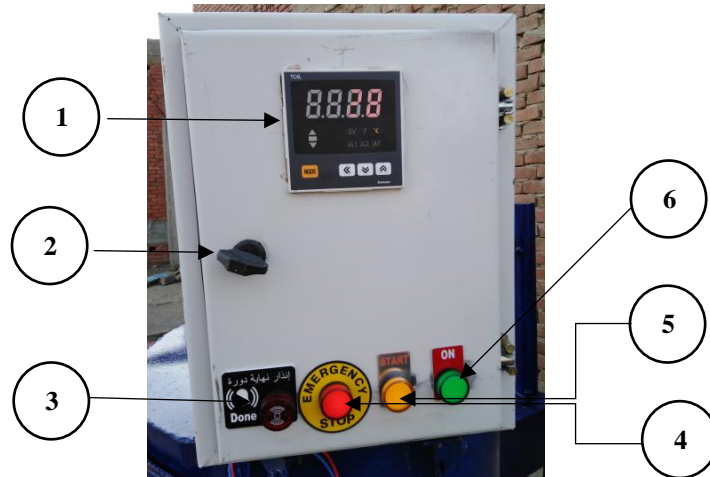
(1) Thermometer, (2) button, (3) alarm, (4) heater lamp, (5) motor lamp and (6) power lamp.
