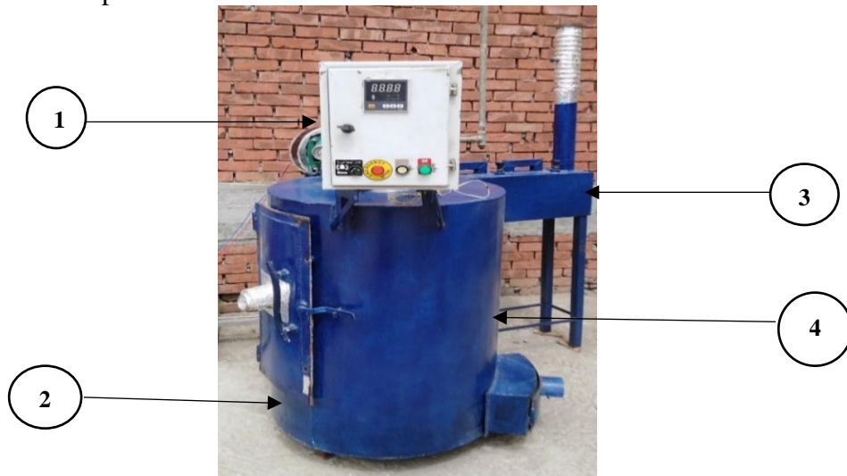
(1) Control unit, (2) fire chamber, (3) treatment unit and (4) carbonization chamber.
