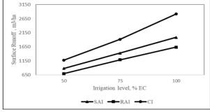
Figure 2. The effect of irrigation level on surface runoff
