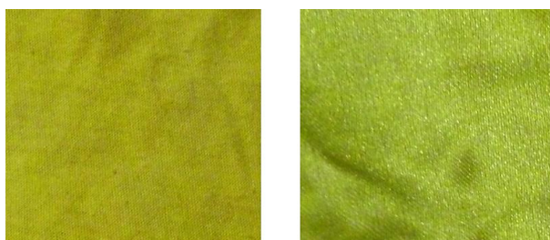
Fig (7): Cotton (left) and silk (right) fabric dyed with turmeric by using aloe vera mordant
