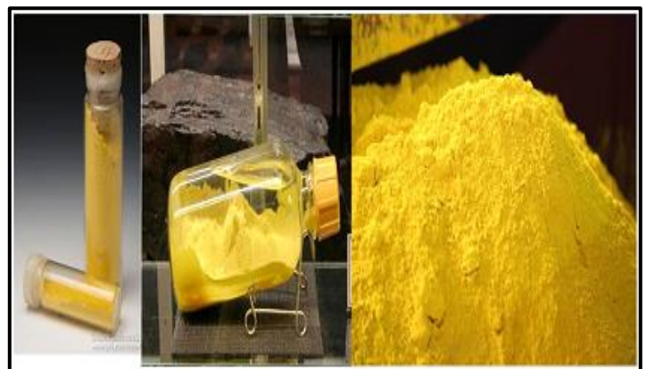
Fig. (1): The uranium solution from the mines is then separated, filtered and dried to produce uranium oxide concentrate, often referred to as “Yellowcake”
