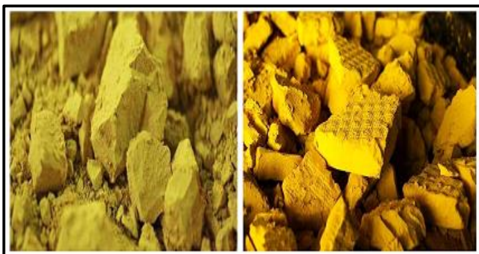
Fig. (2): Yellowcake uranium, a solid form of uranium oxide produce from uranium ore
