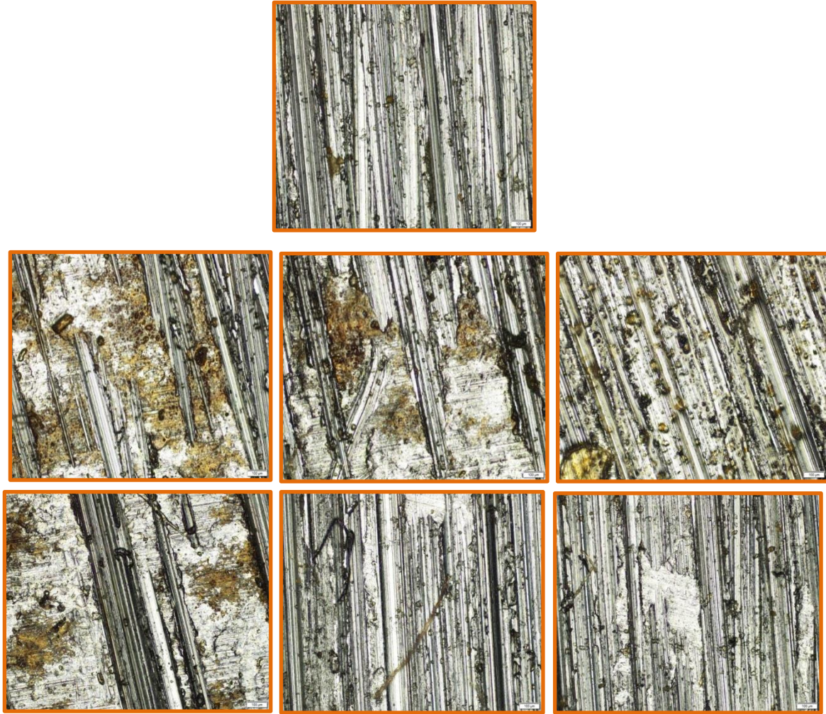
Figure 14. Microscopic images of the worn surfaces of steel surface lubricated by grease dispersing by polymeric additives PE, PTFE and PMMA. Under negative DC current.
