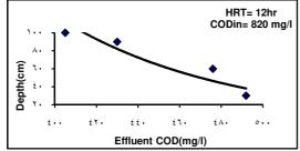
Fig. (9): Effluent COD vs. the Depth of The filter (3<sup>rd</sup> run)anaerobic treatment(3<sup>rd</sup>run)anaerobic treatment
