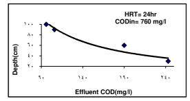
Fig. (5): Effluent COD vs. the Depth of The filter
