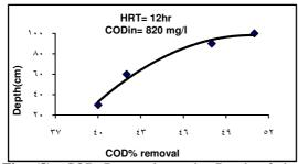
Fig. (8): COD Removal vs. the Depth of the Filter
