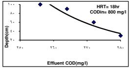
Fig. (7): Effluent COD vs. the Depth of The filter
