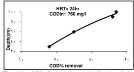
Fig. (4): COD Removal vs. the Depth of the Filter
