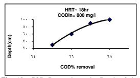
Fig. (6): COD Removal vs. the Depth of the Filter
