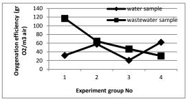
Fig. (6): Relationship between oxygenation efficiency with mixing intensity and air flowrate
