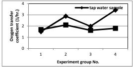
**Fig. (3):** Relationship between oxygen transfer rate with mixing intensity and air flowrate
