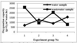
**Fig. (5):** Relationship between oxygenation capacity with mixing intensity and air flowrat
