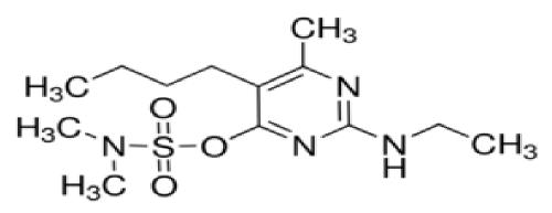
IUPIC name: 5-butyl-2-ethylamino-6-methylpyrimidin-4-yl dimethyl sulfamate Chemical class: pyrimidine Molecular weight: 316.4 Trade name: Nimrod 25% EC CAS No.: 41483-43-6
