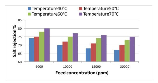
Figure 8:Salt rejection and feed concentration at different temperature values, flow rate = 1 L/min, and vacuum pressure =0.4 bar
