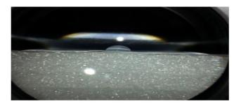
Figure (4) water droplet in contact angle measurement.
