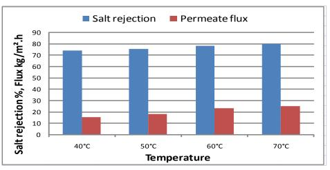
Figure9: Salt rejection and permeate flux at different temperature values, flow rate, vacuum pressure and salt concentration = 5000 ppm.
