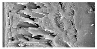
Figure (3) Crosssection of the Membrane
