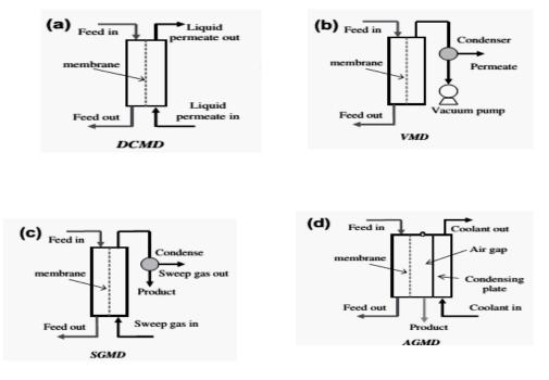
Figure (1) the configurations of the MD (http://emis.vito.be/techniekfiche).
