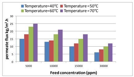
Figure 7Relation between permeates flux and feed concentration at different
