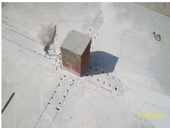
Figure (5) Slab specimen after holes drilling process
