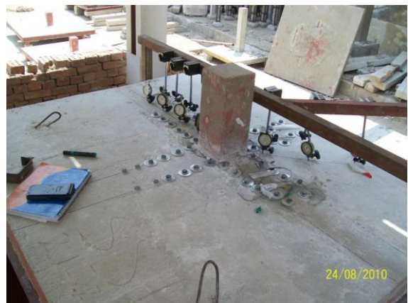
Figure (6) Slab specimen after the installation process of shear bolts
