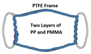
Fig. 6 Framing the mask by PTFE.
