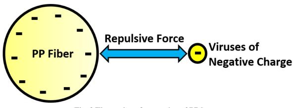
Fig. 3 Illustration of protection of PP layer.
