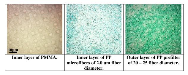
Fig. 2 Optical microscopes of the proposed material for the face mask.
