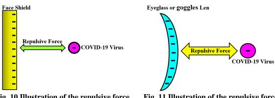
Fig. 10 Illustration of the repulsive force between the face shield and negatively charged viruses.
