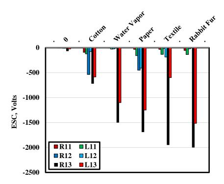
Fig. 9 ESC generated on the surface of the lenses of goggles after rubbing by different materials.
