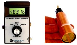
Fig. 1 Electrostatic field measuring device.
