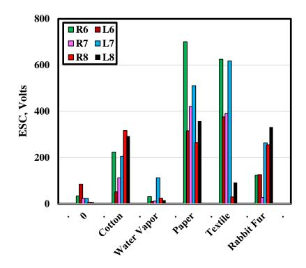
Fig. 7 ESC generated on the surface of the lenses of goggles after rubbing by different materials.
