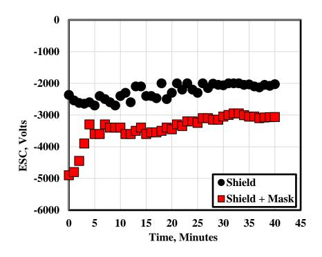
Fig. 3 ESC generated on the surface of face shield versus time.
