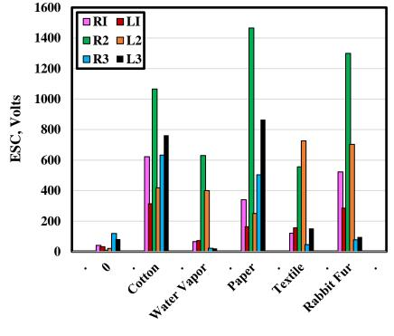
Fig. 5 ESC generated on the surface of the lenses of goggles after rubbing by different materials.
