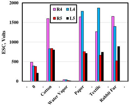
Fig. 6 ESC generated on the surface of the lenses of goggles after rubbing by different materials.
