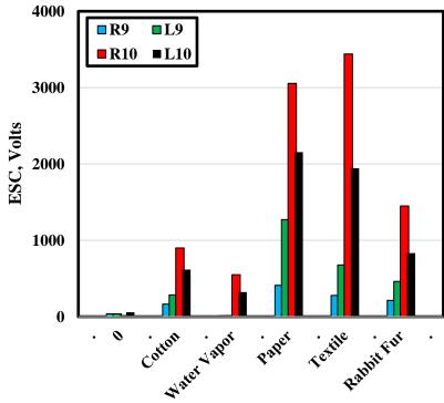
Fig. 8 ESC generated on the surface of the lenses of goggles after rubbing by different materials.
